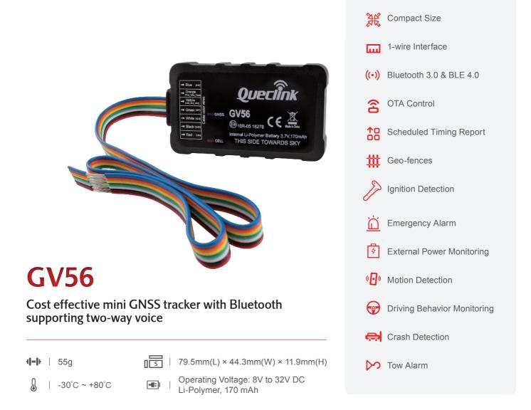
The GV56 is our most cost-effective product for use in light vehicle tracking applications including usage-based insurance, car rental, stolen vehicle recovery, logistics and more. The GV56 optimizes the available I/Os, allowing fuel cut-off, ignition detections, and a single analog sensor in addition to driver ID identification over 1-wire or BLE. Supported accessories include a range of BLE-based fuel and weight monitoring solutions offered from our partners.
